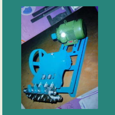
High Pressure Triplex Pumps
