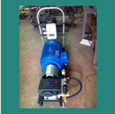
Hydro Test Pump
