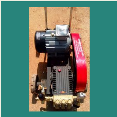
Hydraulic Test Pumps
