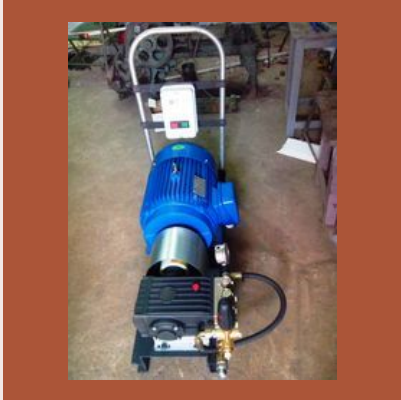
Hydro Test Pump
