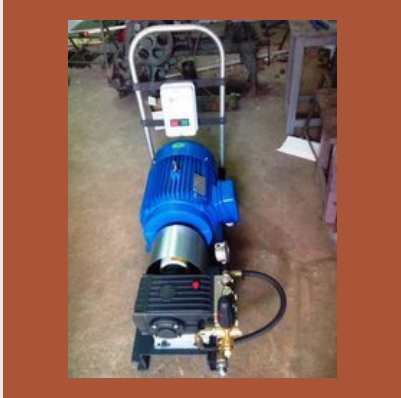
Hydro Test Pump
