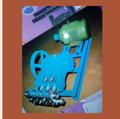
High Pressure Triplex Pumps
